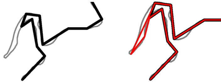
Figure 1. The chopping effect of VW algorithm before (left) and after using partition.
