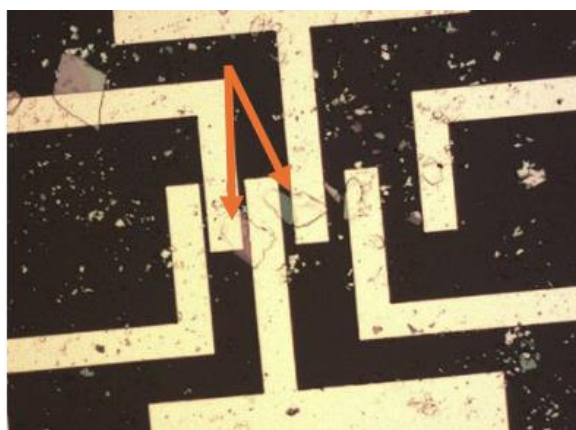
Figure 2:2 a portion of one of our devices. Two 2D semiconductor flakes can be seen at the centre of the image.
